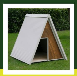
The dog house Shepherd model is made of marine plywood 1,5 cm thick, and has insulated panels for the roof of 3.5 cm thickness, framed with sheet metal profiles. The Cabin has a fixed wooden inner bench, raised from the ground about 7 cm with plastic feet. The entrance is 30 x 44h and is edged with metal antibiting.
